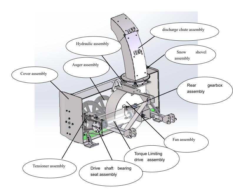
The snow blower is connected to the tractor by a three-point suspension, and the PTO drive shaft of the tractor drives the gear box to work. Through the gear drive, on the one side, the chain drive is driven to Auger weldment and start to work. On the other side, the fan assembly works to suck the surrounding snow into the discharge port. So as to complete the snow removal operation.
