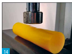
Shock absorber under 25 tonnes pressure retains its shape and properties
