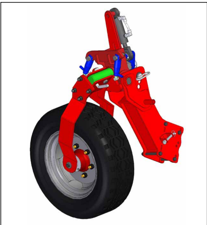
Side transport & support wheel with shock absorber
