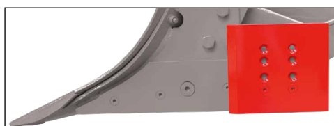
Sliding plate (additional sliding plate). One pair or one piece in standard configuration, depending on plough body type
